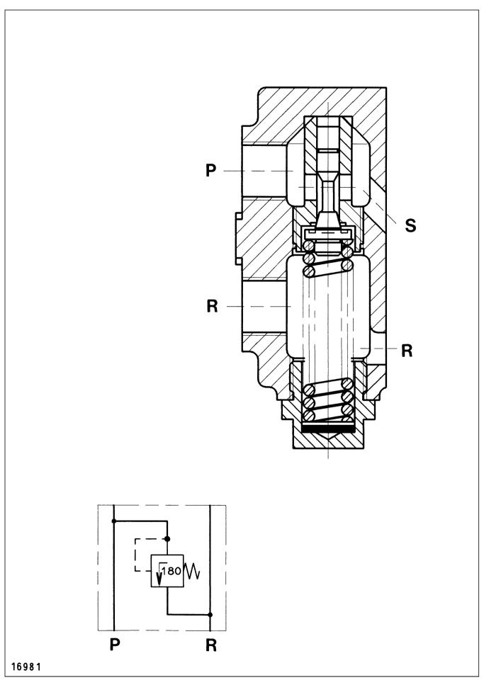
Pressure relief valve Spring-loaded seated valve with damping, directly controlled.
