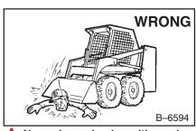
Never leave loader with engine running or with lift arms up.
