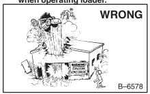
Do not use loader in atmosphere with explosive dust or gas or where exhaust can contact flammable material.
