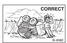
Never loader without operator cab with ROPS and FOPS approval. Fasten your seat
