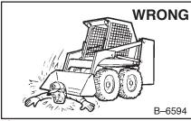
Never leave loader with engine running or with lift arms up.
