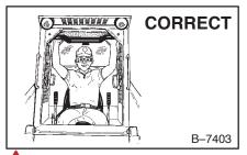
Always use the seat bar and Always keep feet on the foot pedals or footrests when operating loader.
