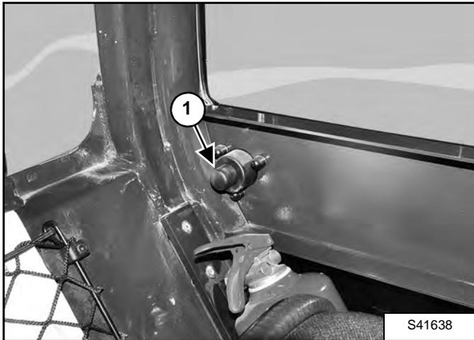
Push the knob (Item 1) [Figure 10-20-4] inside the cab to disengage the latch and close the window.
