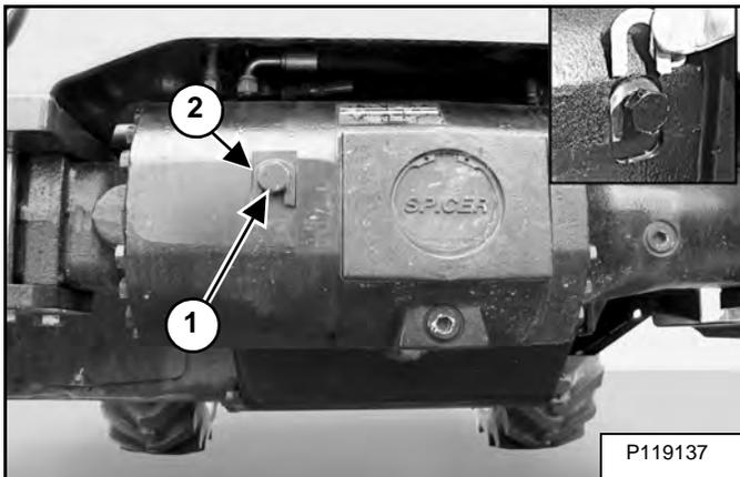
Loosen the two bolts (Item 1) (the bolts and spacers are located on both the front and rear side of the front axle) until the slotted spacers (Item 2) [Figure 10-40-1] can be removed from under the bolt heads.
