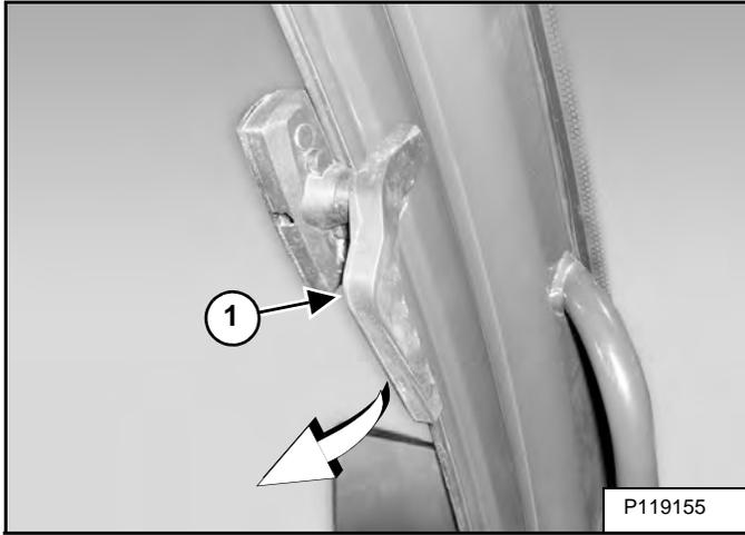
Turn the handle (Item 1) [Figure 10-20-3] (as shown) to unlock the window. Push the window fully open until it latches against the cab.
