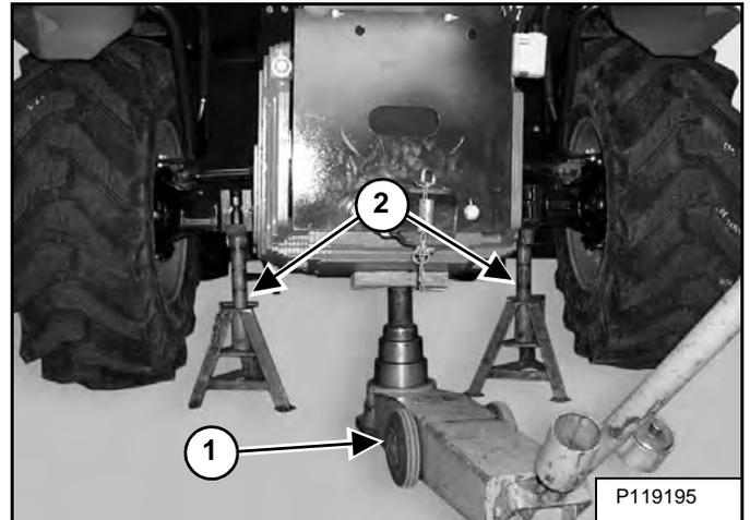
Put the floor jack (Item 1) under the center of the rear weight. Lift the telescopic handler and install jackstands (Item 2) [Figure 10-10-3].
