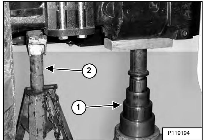
Put the floor jack (Item 1) under the right side of the front axle. Lift the telescopic handler and install the second jackstand (Item 2) [Figure 10-10-2].
