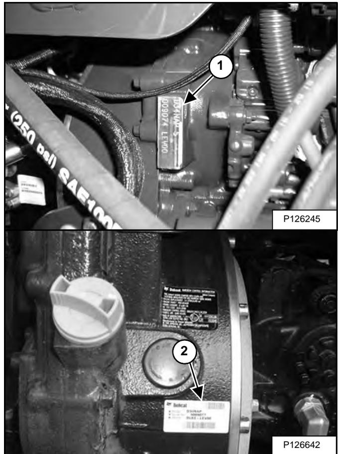
The engine serial number can be found on the engine cylinder block (Item 1) and on the engine rating plate (Item 2) [Figure 2] near the flywheel in front of you when opening the engine cover. Always use the full number (type + number) when ordering replacement parts.
