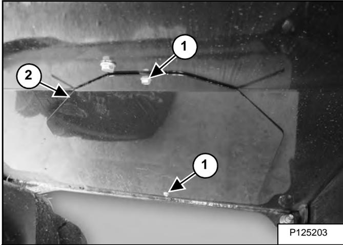
For models TL26.60D(A)(B) and TL30.60(D)(H)B, loosen the two bolts (Item 1) and remove the cover (Item 2) [Figure 10-40-3] from the front side of the engine / hydrostat assembly.
