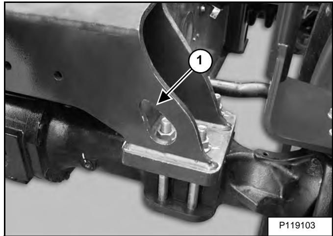
For models not equipped with a front hitch, use the two front transportation fastening points (Item 1) [Figure 10-40-8] and [Figure 10-40-9] for towing.
