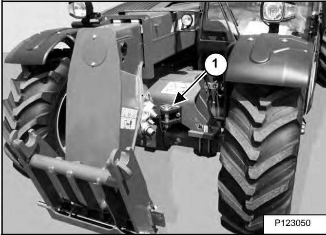
Use the front hitch (if equipped) (Item 1) [Figure 10-40-7] for towing.
