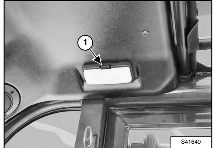
The cab light [Figure 10-20-8] is located above the operator's left shoulder.
