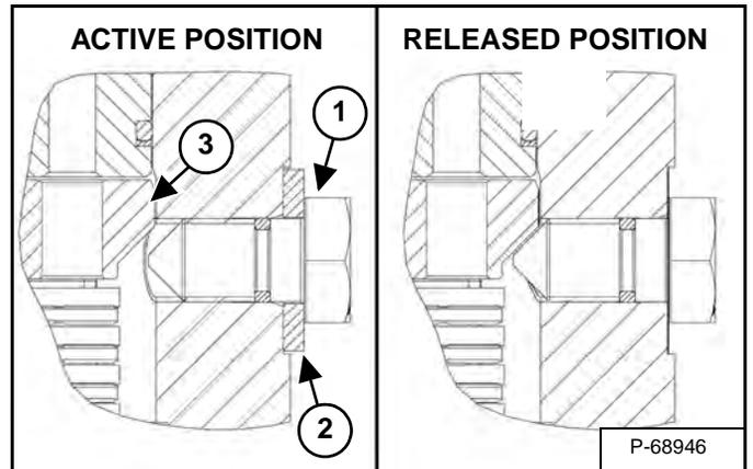
Evenly tighten the front and rear bolts (Item 1) to hold the spacers (Item 2) [Figure 10-40-5] and [Figure 10-40-6].
