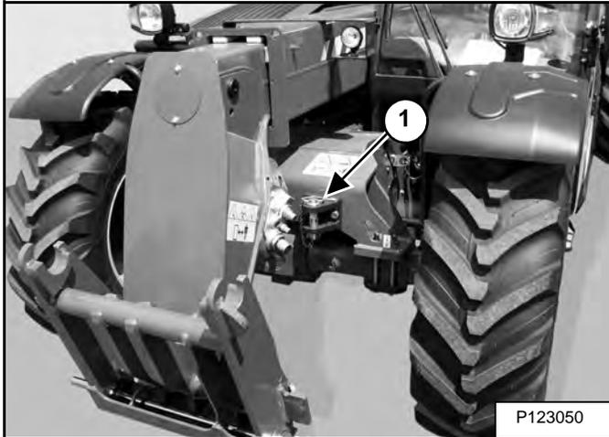
Use the front hitch (Item 1) [Figure 10-40-10] for retrieval of machine out of a hole or ditch.
