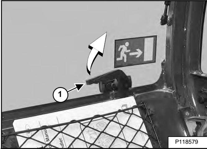
Turn the handle (Item 1) [Figure 10-20-6] (as shown) to unlock the rear window.
