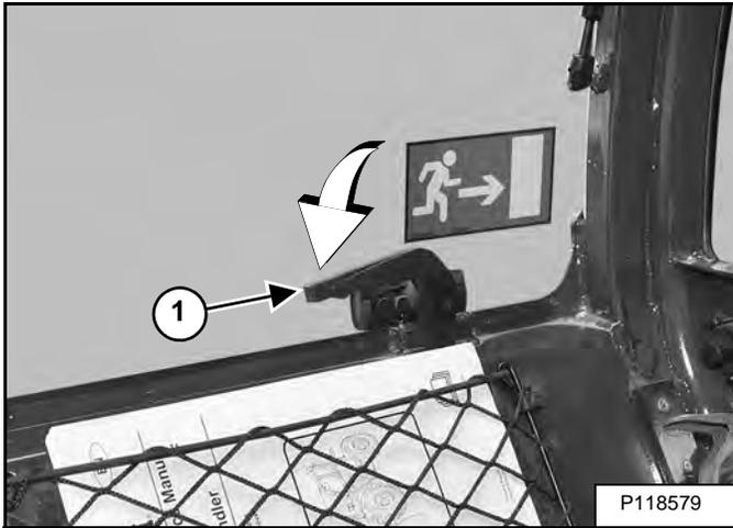
Turn the handle (Item 1) [Figure 10-20-7] back into the original position (as shown) to lock the window.
