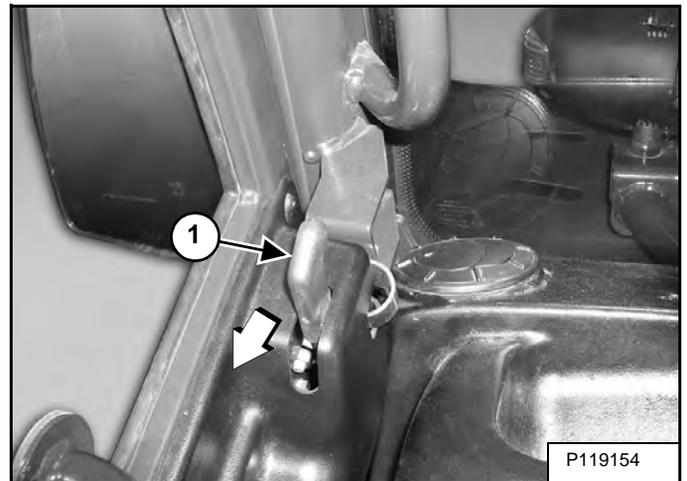
The cab door can be opened from the outside of the cab using the latch (Item 1) [Figure 10-20-1] and opened from the inside of the cab when you pull the lever (Item 1) [Figure 10-20-2] back (as shown).
