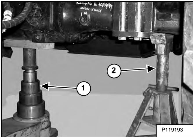
STOP the engine. Put the floor jack (Item 1) under the left side of the front axle. Lift the telescopic handler and install the first jackstand (Item 2) [Figure 10-10-1].
