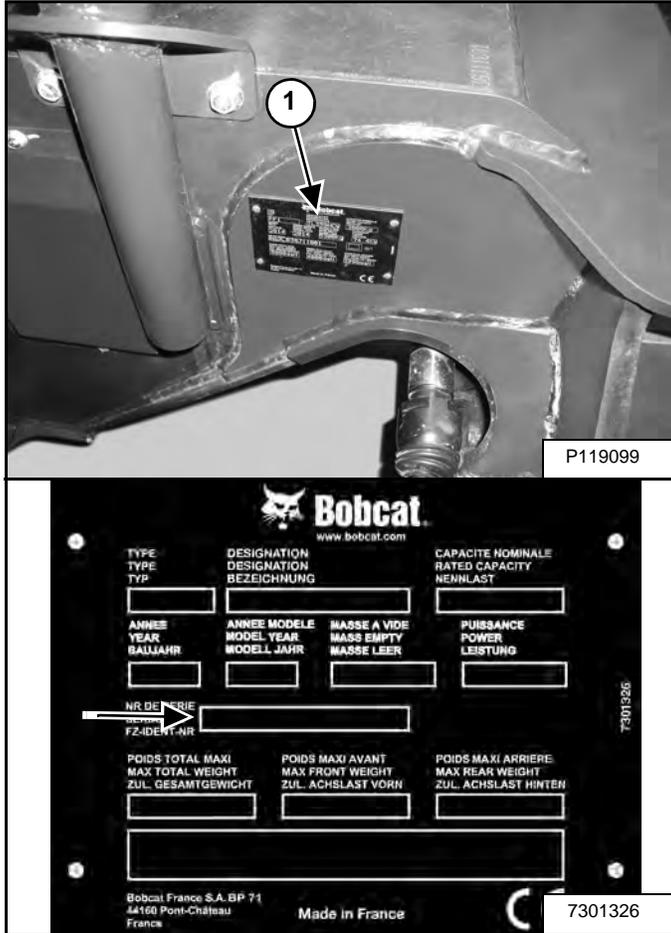
The telescopic handler serial number plate (Item 1) is located on the right side of the chassis in front [Figure 1].
