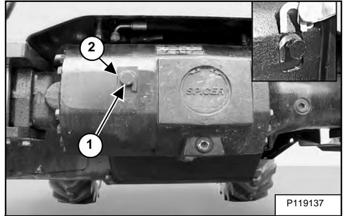
Loosen the two bolts (Item 1) until the spacers (Item 2) [Figure 10-40-5] can be installed under the bolt heads (the bolts and spacers are located on both the front and rear side of front axle).
