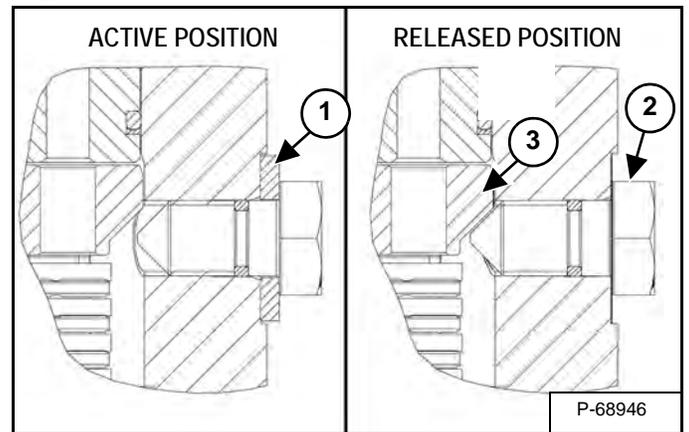
After removing the spacers (Item 1), evenly tighten the front and rear bolts (Item 2) to hold the parking brake piston (Item 3) [Figure 10-40-2] in the released position.
