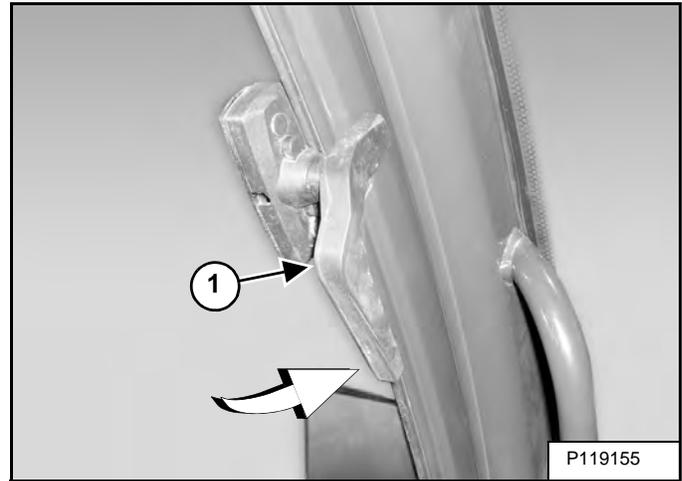
Turn the handle (Item 1) [Figure 10-20-5] back into the original position (as shown) to lock the window.
