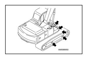
If grasping the door handrail when mounting or dismounting or moving on the track, open and lock the door securely in the open position. Otherwise, the door may move suddenly, causing you to lose balance and fall.
