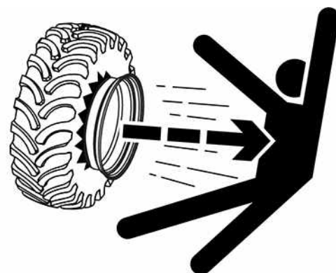
RXA0103438-UN: Explosive Tire and Rim Parts
