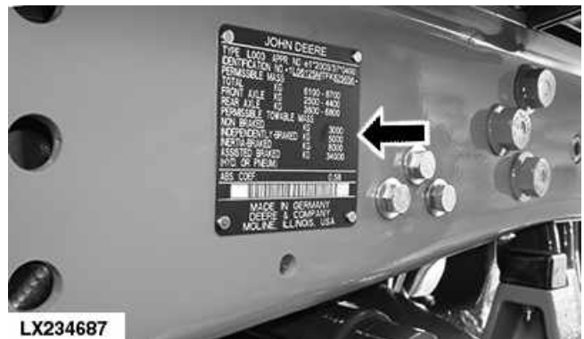
LX234687-UN: Position of the Type Plate with the Tractor Serial Number
