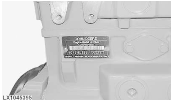
LX1045395-UN: Engine serial number
