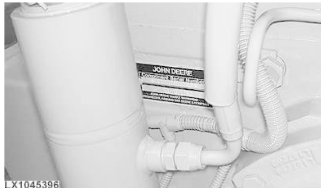
LX1045396-UN: Transmission Serial Number
