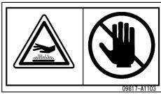
Sign indicates a burn hazard from touching heated parts, such as engine, motor, or muffler during or right after operation.
