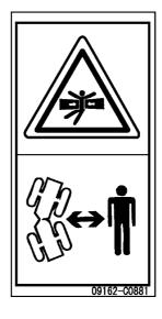
Sign indicates a crush hazard between the articulating parts of vehicle.
