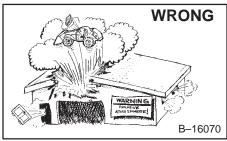
Do not use machine in atmosphere with explosive dust or gas or where exhaust can contact flammable material.
