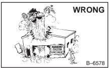
Do not use loader in atmosphere with explosive dust or gas or where exhaust can contact flammable material.
