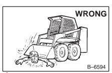
Never leave loader with engine running or with lift arms up. To park, engage parking brake
