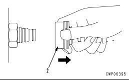
Hold the mouthpiece of the tightening portion and push body (2) in straight until sliding prevention ring (1) contacts contact surface a of the hexagonal portion at the male end to connect it.
