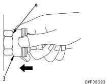
B) Hold in the condition in Steps 1) and 2), and pull out whole body (2) to disconnect it.
