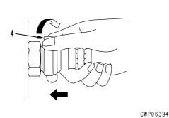
3) Hold in the condition in Steps 1) and 2), and pull out whole body (2) to disconnect it.
