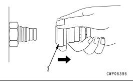
Hold the mouthpiece of the tightening portion and push body (2) in straight until sliding prevention ring (1) contacts contact surface a of the hexagonal portion at the male end to connect it.
