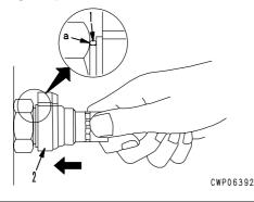
Hold the mouthpiece of the tightening portion and push body (2) in straight until sliding prevention ring (1) contacts contact surface a of the hexagonal portion at the male end.
