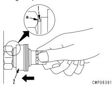
Hold in the condition in Step 1), and push until cover (3) contacts contact surface a of the hexagonal portion at the male end.
