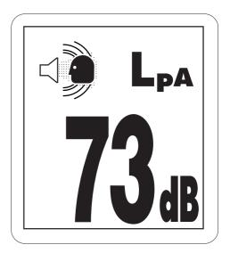
Sound power level emitted by the machine, measured according to ISO 6395 (Dynamic test method, simulated working cycle). This is the guaranteed value as specified in European directive 2000/14/EC.
