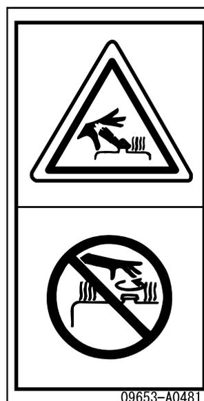
Sign indicates a burn hazard from spurting hot water or oil if radiator or hydraulic tank is uncapped while hot.
