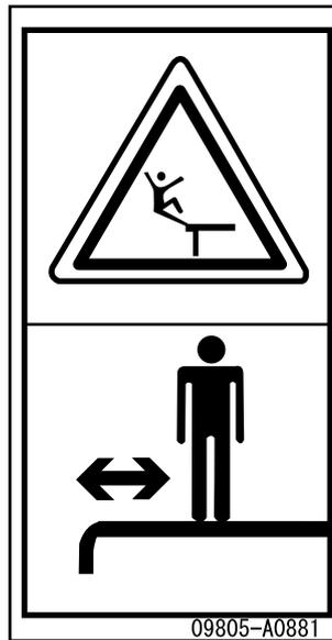
Sign indicates a hazard of falling off the fender or hood.
