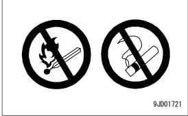
When performing grinding or welding work on the machine, move any flammable materials to a safe place before starting.
