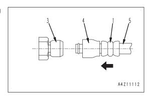
After inserting the hose in the mating adapter perfectly, pull it back to check the connecting condition.
