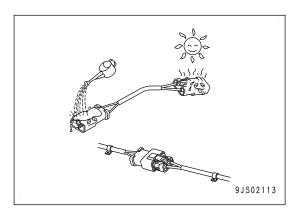
If AdBlue/DEF is spilled over wiring harness and connectors, it may cause corrosion and defective contact.
