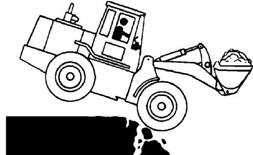
Operate Only on Solid Footing
