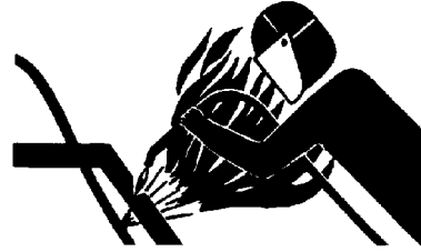
Heating Near Pressurized Fluid Lines
