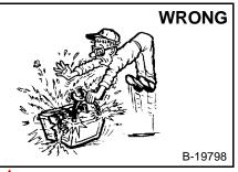
produce Lead-acid batteries flammable and explosive gases.
