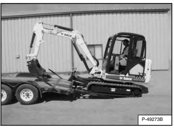
Move the machine forward onto the transport vehicle [Figure 10-30-1].
