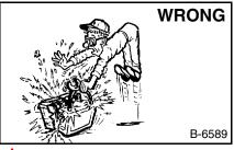
Lead-acid batteries produce flammable and explosive gases.
