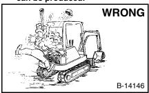
Stop, cool and clean engine of flammable materials before checking fluids.
