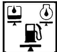
14. Inspect for fuel, oil or hydraulic fluid leaks.
