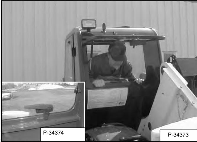
Turn the handle (Inset) and push the rear window open. Exit through the rear window opening [Figure 10-20-1].
