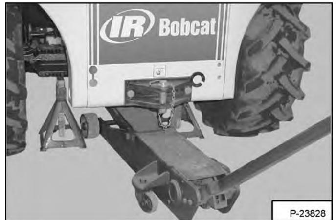
Put the floor jack under the center of the rear axle. Lift the Versa HANDLER and install jackstands [Figure 10-10-2].
