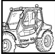
2. Check that ROPS mounting hardware is tightened and is Bobcat approved.
