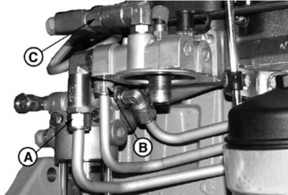
Final Fuel Filter Fuel Lines
