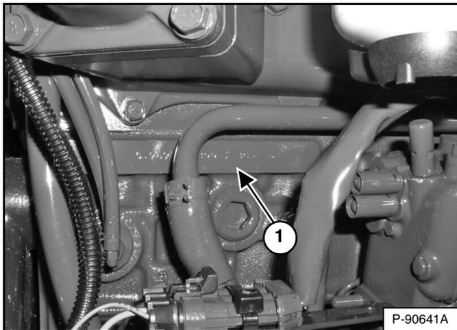
The engine serial number (Item 1) [Figure 2] is located on the side of the engine above the oil filter.
