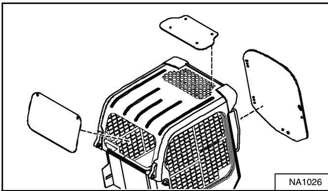
Available for special applications to restrict material from entering cab openings. Kit includes 12,7 mm (0.5 in) thick polycarbonate front door and polycarbonate rear window [Figure 4].
