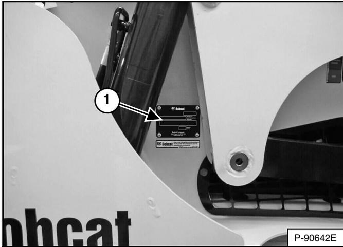
The loader serial number plate (Item 1) [Figure 1] is located on the outside of the loader frame.
