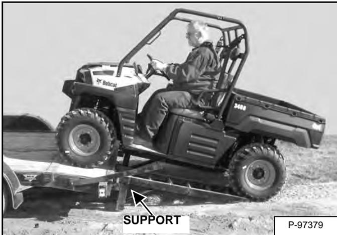
The Utility Vehicle can be loaded or unloaded forward or backward [Figure 10-30-1].
