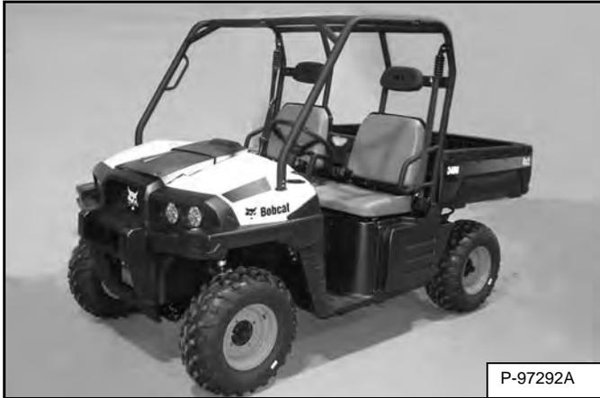
The 3400 and 3400XL have a Rollover Protective Structure (ROPS) to provide protection from rollover [Figure 10-20-1]. The seat belt must be worn for rollover protection.
