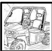
2. Check that ROPS mounting hardware is tightened and is Bobcat approved.
