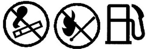
Stop the engine and let it cool before adding fuel. No smoking! Do not refuel a utility vehicle near open flames or sparks. Fill the fuel tank outdoors.
