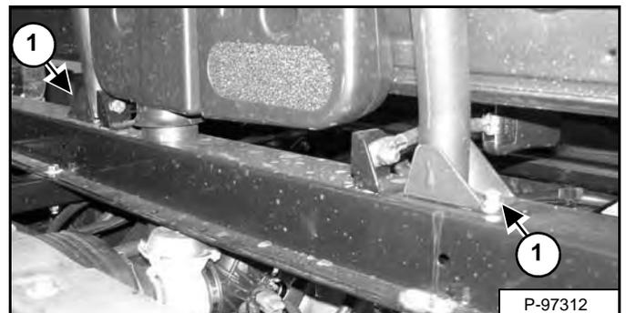
The correct torque for ROPS to frame mounting hardware (Item 1) [Figure 10-20-4] is 20 - 24 N•m (16 - 18 ft-lb).
