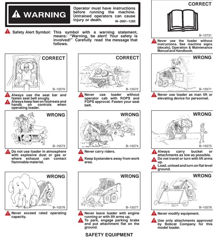
The Bobcat loader must be equipped with safety items necessary for each job. Ask your dealer for information on the safe use of attachments and accessories.
