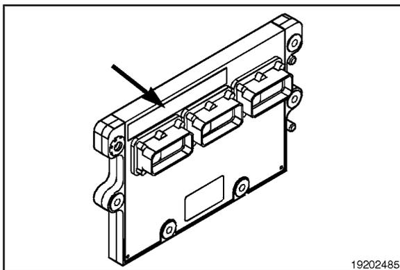
The CM570 is the fuel control module for the engine.
