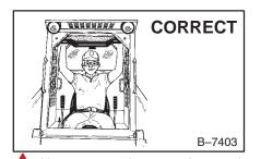
Always use the seat bar and fasten seat belt snugly. Always keep feet on the foot footrests pedals or when operating loader.
