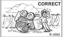
Never loader without use operator cab with ROPS and FOPS approval. Fasten your seat belt.
