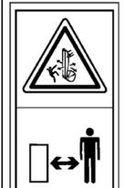
Sign indicates a hazard of being hit by the working device of the machine.
