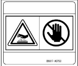
Sign indicates a burn hazard from touching heated parts, such as engine, motor, or muffler during or right after operation.
