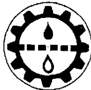
Fig. 6-Transmission Oil Filter Indicator Light
