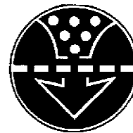
Fig. 49-Air Filter Indicator Light
