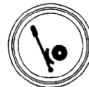
Fig. 10-Parking Brake Indicator Light
