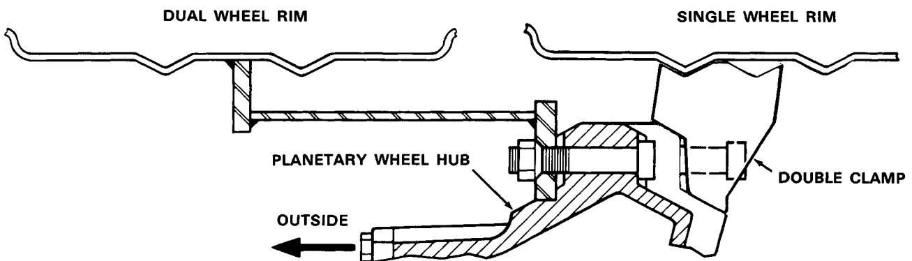
For the 18.4 x 30 or 18.4 x 34 dual wheel tread spacing, the inner wheels and tires must be set at the 72" tread spacing. Then when the outer dual wheels and tires are installed, the proper running clearance between the tires will be reached.
