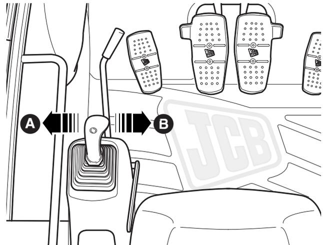
Before slewing the cab, ensure that the slew lock is switched off (see **Facia Panel**).
