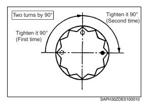
(3) Tightening method after tightening to seating torque
