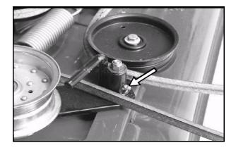
There are two grease fittings for the deck raising pivot bushings - one on each side of the unit.
