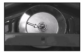
There is a grease fitting for the deck idler arm bushing.
