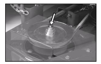
The grease zerk for the center mower spindle.
