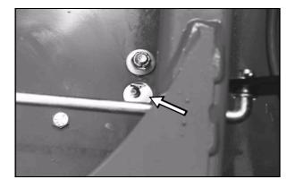
Also under the seat are the fittings for the motion control lever pivot bushings - one for each lever.
