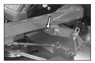
The grease zerk for the deck height adjustment lever is on the right side of the machine.
