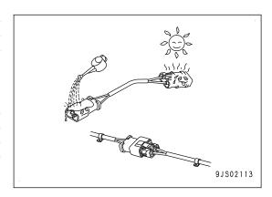
If DEF is spilled over wiring harness and connectors, it may cause corrosion and defective contact. Be careful not to spill it over electrical equipment, wiring harness and connectors since DEF is strongly corrosive to metal.
