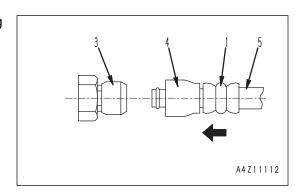
2. After inserting the hose in the mating adapter perfectly, pull it back to check the connecting condition.
