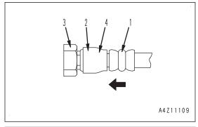
2. While having adapter (3) inserted into hose side joint (2), insert rubber cap (4) to adapter (3) side until it clicks.
