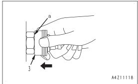
3. While keeping the conditions of steps 1 and 2, pull out whole body (2) to disconnect it.
