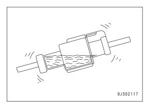
If any water, mud or dust is stuck to the outside surface of a connector, it can enter inside the connector when the connector is disconnected. Before disconnecting the connector, wipe off any stuck water or dirt by using a dry cloth or blow it with compressed air.
