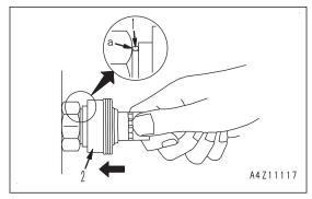
2. While keeping the condition of step 1, push cover (3) straight until it contacts contact surface (a) of the hexagonal portion on the male side.
