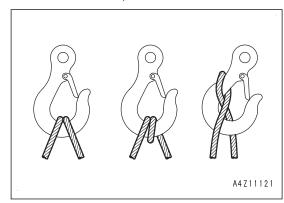
Never use a wire rope which has breaks in strands (A), reduced diameter (B), or kinks (C). There is a danger that the rope may break during the towing operation.
