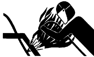
Heating Near Pressurized Fluid Lines
