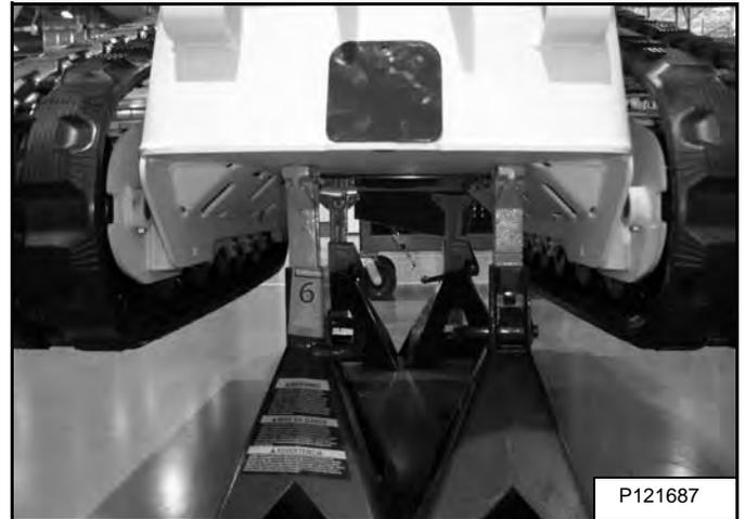
Raise the front and rear of the machine and put jackstands under each corner [Figure 10-10-2]. Lower the machine to the jackstands.
