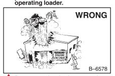
Do not use loader in atmosphere with explosive dust or gas or exhaust where can contact flammable material.
