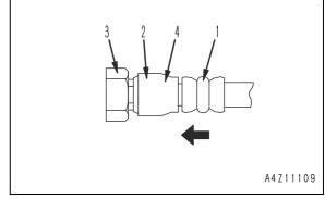
2. While you have the adapter (3) engaged into hose side joint (2), inner rubber cap (4) to adapter (3), side it in until it clicks.
