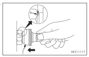
2. While you keep the condition of step 1, push cover (3) straight until it touches surface (a) of the hex part on the male side.
