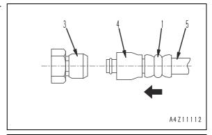
2. After you put the hose in the adapter, pull it to make sure it connected correctly.
