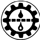
Fig. 22-Transmission Oil Filter Indicator Light
