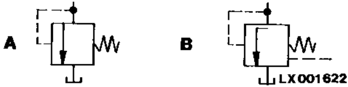
Hydraulic symbols—pressure relief valves
